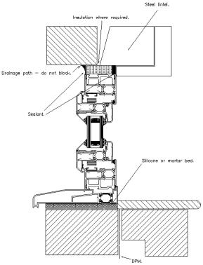
Head arrangement and Sub-sill arrangement
